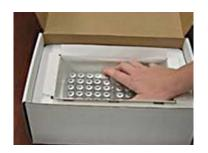
Load product in the chamber, replace cooling lid, close the container and tape shut.
